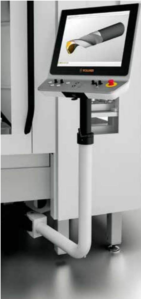
///// CONTROL DESK High-quality LCD display with touchscreen and multifunction handwheel
